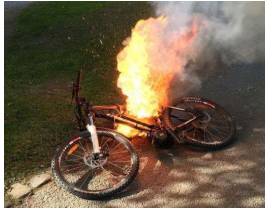
Li-ion bike fire during use. http://i.imgur.com/QexArU9.jpg
