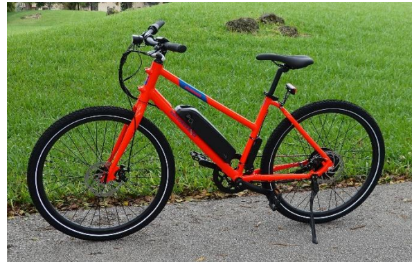
Typical budget e-bike, note battery pack on bike frame.
